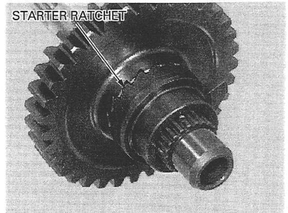
Remove the snap ring, washer and starter pinion gear from the spindle.
