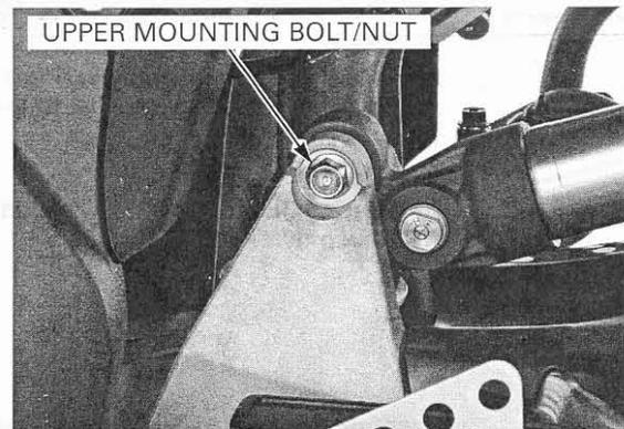
Install the lower mounting bolt and nut. Tighten the upper and lower mounting nuts to the specified torque.
