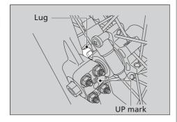
3. Tighten the front axle shaft.
