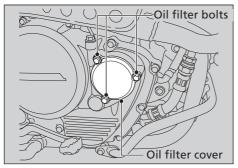
**7.** Check that the oil filter cover O-ring is in good condition.
