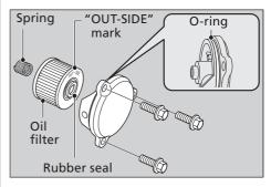
**9.** Install the oil filter cover by tightening the oil filter cover bolts.
