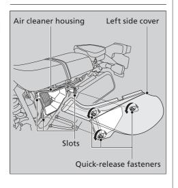
The left side cover must be removed for seat removal, or to service the air cleaner, fuse or battery maintenance.
