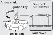
Do not fill with fuel above the plate. **Fuel type:** Unleaded gasoline only Recommended fuel octane number: Pump Octane Number (PON) 86 or higher. **Tank capacity:** 2.77 US gal (10.5 liters) **Reserve capacity:** 0.61 US gal (2.3 liters)
