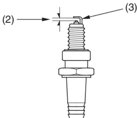
(2) spark plug gap    (3) side electrode
