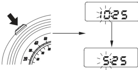
5. Push and hold the odometer/tripmeter/digital clock select and reset button for more than 2 seconds. The minute display will start flashing.
