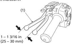
(1) rear brake lever/parking brake lever
