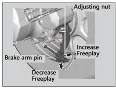
**2.** Apply the brake several times and check for free wheel rotation after the brake lever is released.
