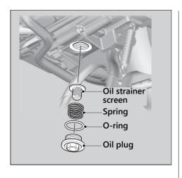
**10.** Install the oil strainer screen, spring and oil plug and tighten.
