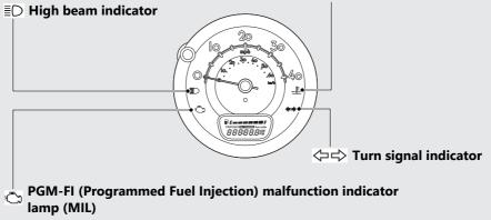
Comes on briefly when the ignition switch is turned to the ON position.
