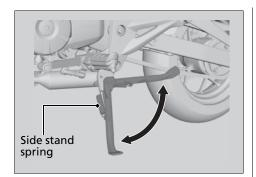
smoothly. If the side stand is stiff or squeaky, clean the pivot area and lubricate the pivot bolt with clean grease.
