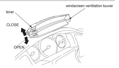
You can adjust the windscreen ventilation louver with the lever to control and direct the flow of fresh air
