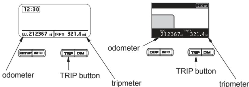
The tripmeter will show mileage in two sub modes, “TRIP A” and “TRIP B.” Push the TRIP button to select the “TRIP A” or “TRIP B” mode.
