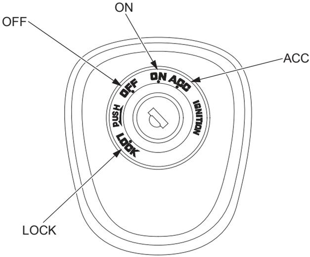
The ignition switch is used for starting and stopping the engine ([page 55](#)) and to lock the steering for theft prevention ([page 65](#)). Insert the key and turn it to the right for the ON and ACC (accessory) positions. Push down on the key and turn it to the left to the LOCK (steering lock) position.
