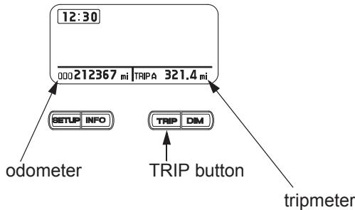
The tripmeter will show mileage in two sub modes, “TRIP A” and “TRIP B.” Push the TRIP button to select the “TRIP A” or “TRIP B” mode.
