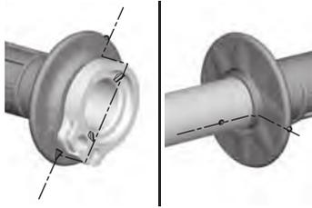
For added security, you may choose to bind the handgrips to the handlebar and throttle pipe with safety wires to prevent the possibility of them loosening. Position the twisted wire ends away from your palms and be sure to bend the wire ends well into the handgrip rubber so they will not snag your glove.
