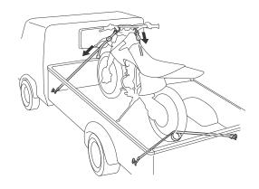
To secure your motorcycle, brace the front wheel against the front of the truck bed or trailer rail. Attach the lower ends of two straps to the tie-down hooks on your vehicle. Attach the upper ends of the straps to the handlebar (one on the right side, the other on the left), close to the fork.
