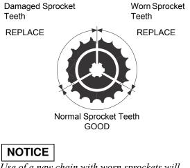
*Use of a new chain with worn sprockets will cause rapid chain wear.*
