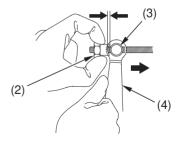
(2) rear brake adjusting nut(3) brake arm pin(4) brake arm
