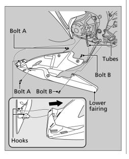
The lower fairing must be removed to change the oil filter.
