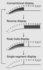
2 Press SET button. The currently selected displaying mode is set, and the control returns to the ordinary display.
