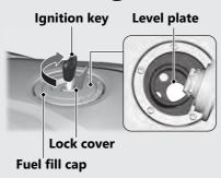
Do not fill with fuel above the level plate. Fuel type: Unleaded gasoline only Recommended fuel octane number: Pump Octane Number (PON) 86 or higher. **Tank capacity:** 4.41 US gal (16.7 L)
