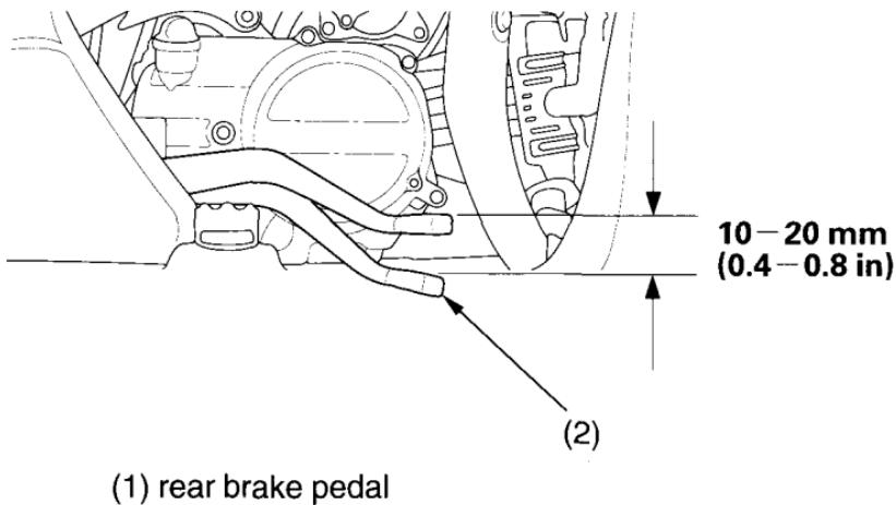
Measure the distance the rear brake pedal (2) moves before the brake starts to take hold. Freeplay, measurement at the tip of the end of the pedal, should be:
