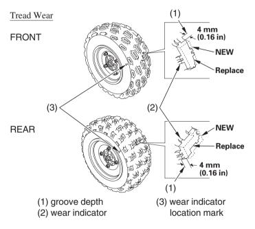
To check the condition of a tyre tread, measure the groove depth (1) in the centre of the tyre, or check the wear indicator (2).
