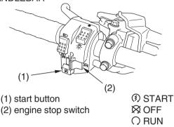
The start button (1) is used for starting the engine. Pushing the button in starts the engine. See *Starting Procedure*, page 50.
