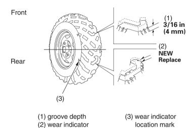
To check the condition of a tire tread, measure the groove depth (1) in the center of the tire, or check the wear indicator (2).
