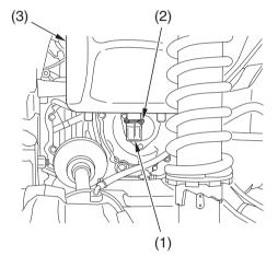
(1) drain tube(3) air cleaner housing(2) clip
