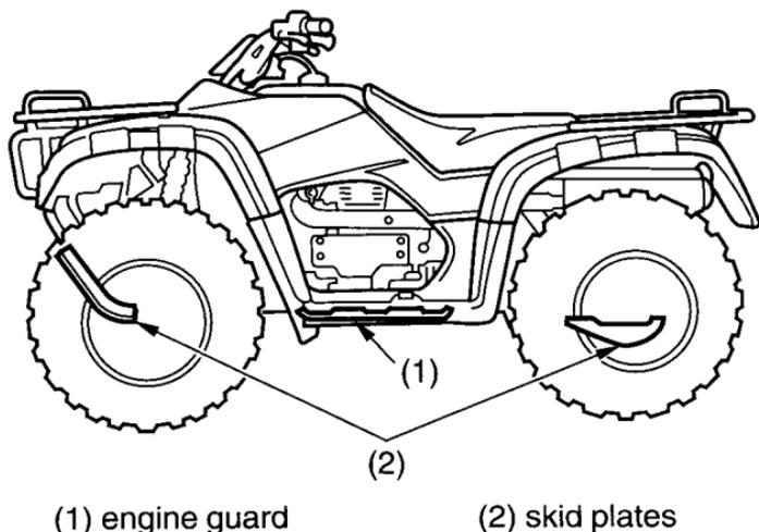
The engine guard (1) protects the engine crankcase.
