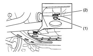
(1) engine oil drain plug (2) sealing washer
