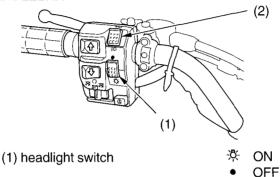
The headlight switch (1) is used to turn the headlight ON ( $^{*}$ ) or OFF ( $^{\bullet}$ ). To operate, turn the switch to ON ( $^{*}$ ) or OFF ( $^{\bullet}$ ).
