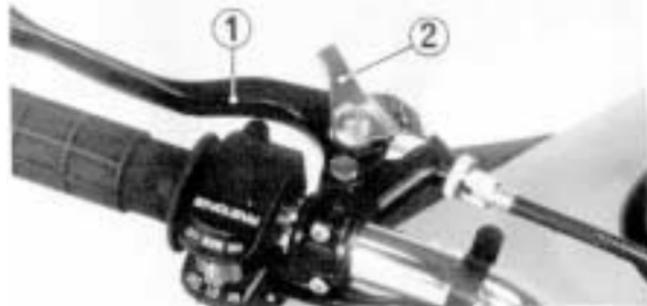
(1) Brake lever/Parking brake (2) Lock
