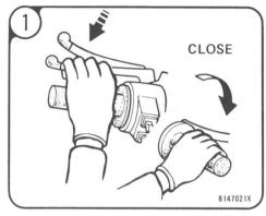
Close the throttle and apply the rear brake when moving the machine off the stand or loss of control may result.
