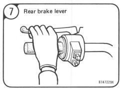
To start the engine, CLOSE THE THROTTLE and apply the rear brake. This will allow the spring to crank the engine for starting.
