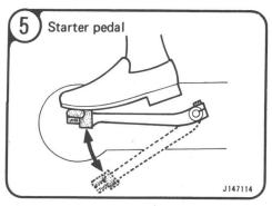
The engine is started by a spring which is tensioned by pressing down the starter pedal three full strokes or untill the positive stop is felt.
