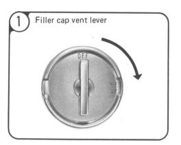
Turn the fuel filler cap vent lever to the "ON" position.
