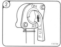
Turn the fuel valve lever to the "ON" position.
