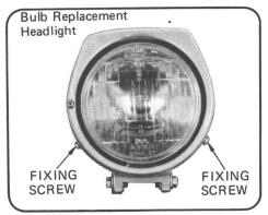
Remove the two headlight fixing screws and remove the headlight from the headlight case.
