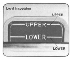
Level must be maintained between the "UPPER" and "LOWER" level marks.
