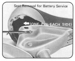
Remove the wing-bolt and push back on the seat to remove.
