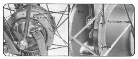
If the arrow aligns with the reference mark on full application of the brake, replace the brake shoes.
