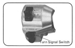
Move to "L" to signal a left turn, "R" to signal a right turn. Return to the center (off) when finished.
