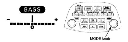
To select the Treble control, push the MODE knob two times, and "TREBLE" will appear on the display. Then, within five seconds, change the treble control.
