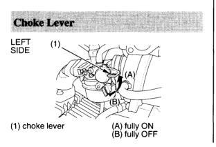
The choke lever is used for starting the engine (page 31). The choke increases the percentage of fuel in the fuel/air mixture delivered to the engine.
