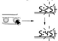
4. Wait approximately 10 seconds; the display will stop flashing automatically. If the ignition switch is turned off during the time adjustment mode, the time adjustment will become invalid. At the same time, the blinking function of the immobilizer system (HISS) indicator will be altered.
